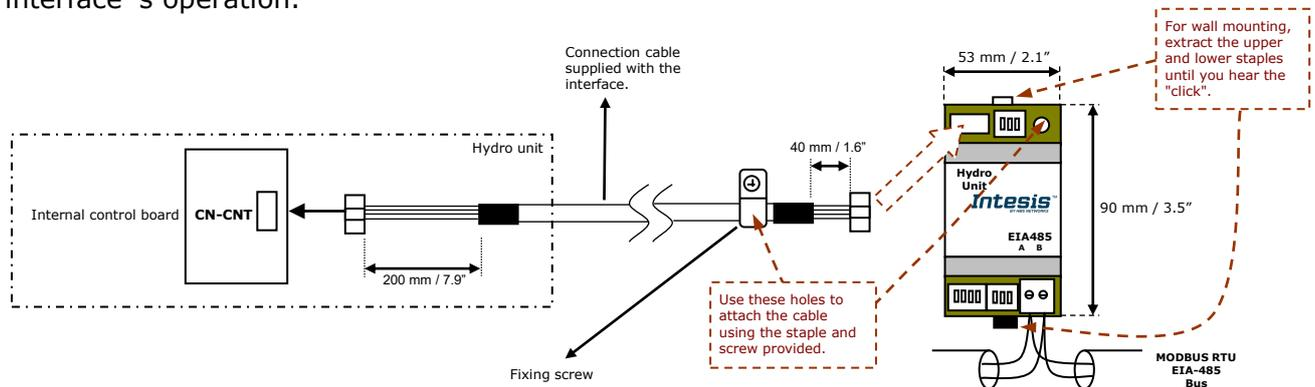
Figure 2.1 INMBSPAN001A000 connection diagram
